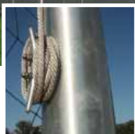
Tie-down cleat prevents the hoisting rope from becoming a tripping hazard.
