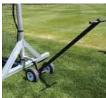
Specially designed hitch attachment with wheels & handle.
